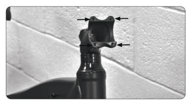
• Place the handlebar into the handlebar stem and screw the 4 bolts in using an allen key.
