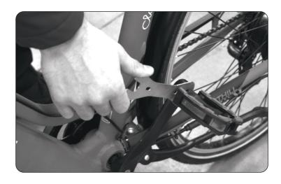
• The right pedal is attached on the same side as the chain. Make sure you check the pedals are tight and secure before riding.
