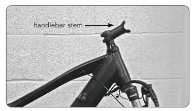
• Unscrew the 4 bolts in the handlebar stem using an allen key.
