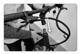
2. Once the stem is in the correct position, tighten the bolt going down through the stem with an allen key ①. Once the bolt is correctly tightened, check if the stem and handlebars are straight with the front wheel. Then tighten bolts ②. Please be careful not to overtighten the bolts.
