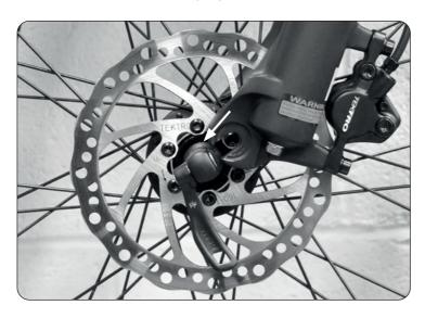
• Tighten the nut and hold the lever in an upright position as shown in the photo below. Once tight push the lever in to secure the wheel.
