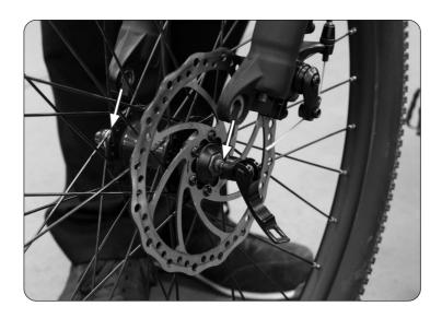
• Tighten the nut and hold the lever in an upright position as shown in the photo below. Once tight push the lever in to secure the wheel.
