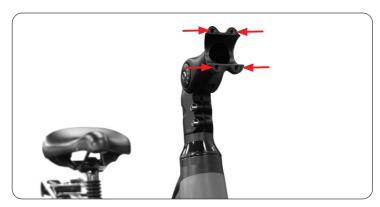
• Place the handlebar into the handlebar stem and screw the 4 bolts in using the provided allen key.
