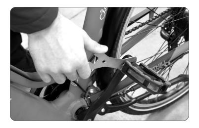
• The right pedal is attached on the same side as the chain. Make sure you check the pedals are tight and secure before riding.
