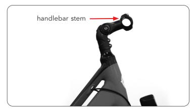
• Unscrew the 4 bolts in the handlebar stem using the provided allen key.
