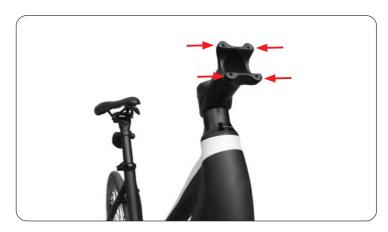
• Place the Handlebar into the Handlebar Stem and screw the 4 bolts in using the provided Allen Key.
