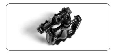
• To connect the Pedals to the bike, place L into the Left tube and R into the Right tube (left and right directions are as though you are sitting on the bike). Tighten by turning the Pedals toward the Front Wheel. Use a wrench to make sure the Pedals are tight and secure.
